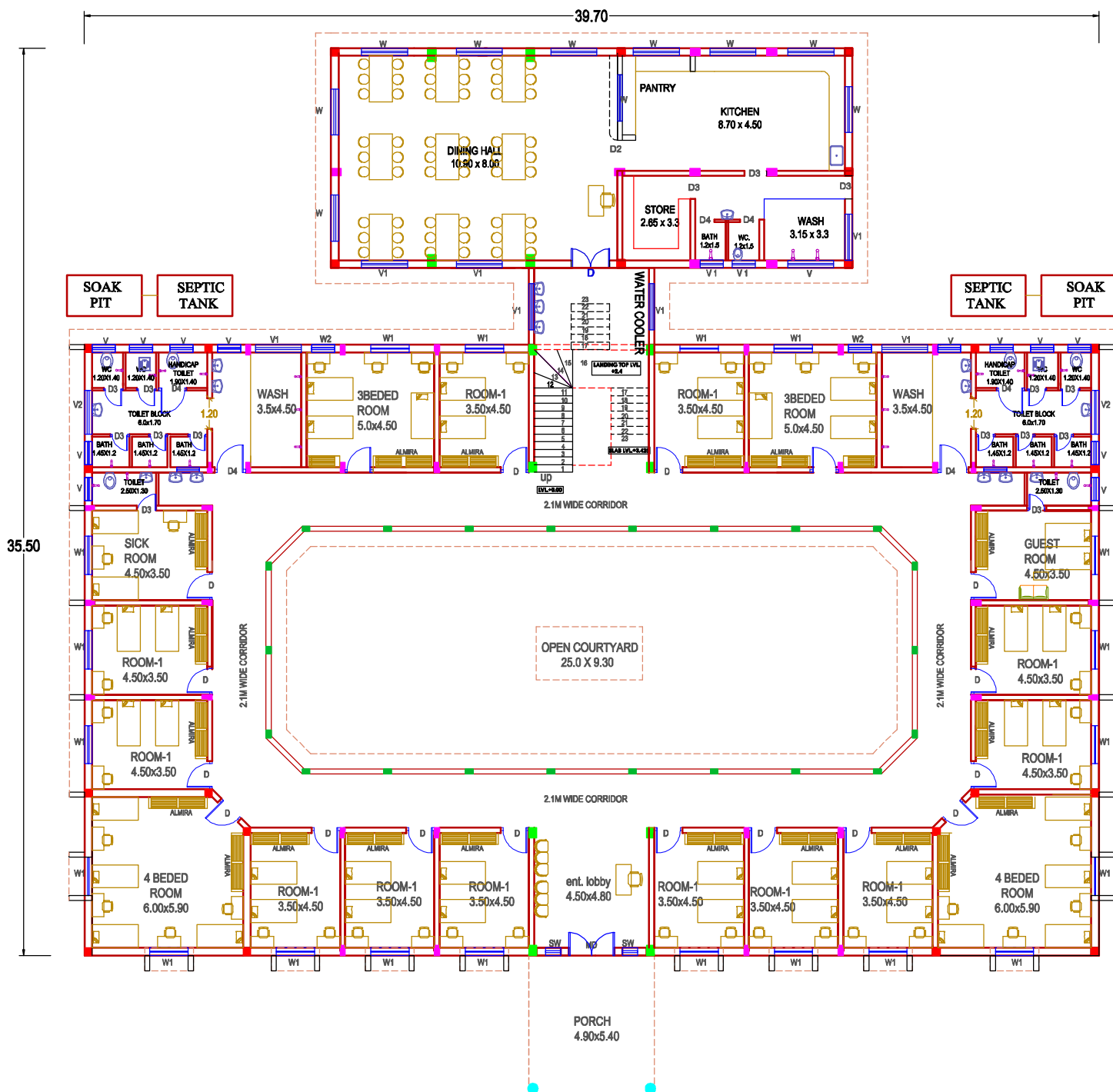
GROUND FLOOR PLAN (BUILT UP AREA - 900 SQM)
